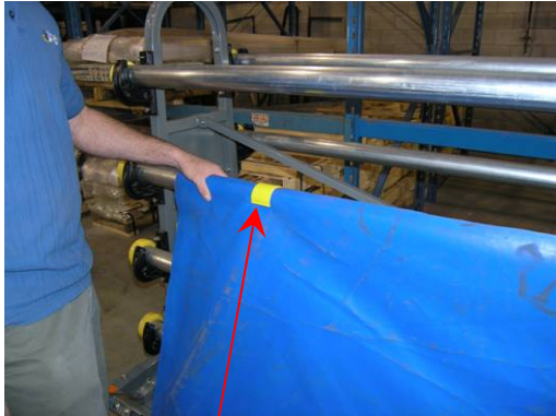
Fig 22.1 Quick-clip on end side of cover
