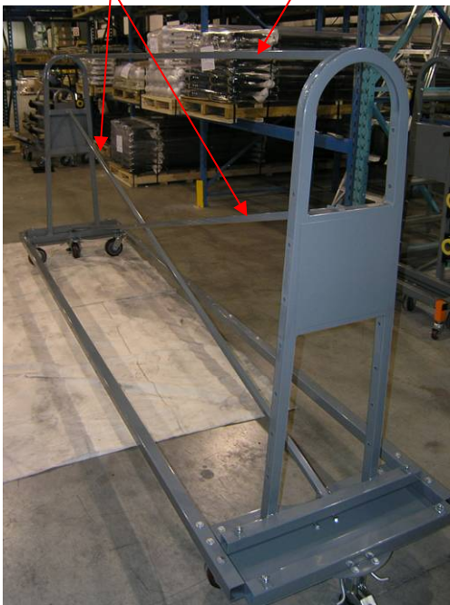
Fig 9.1 Top and Cross Brace Installation
