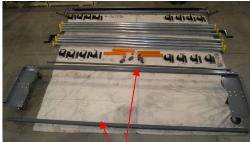
Fig 4.1 Side Rail Sections
