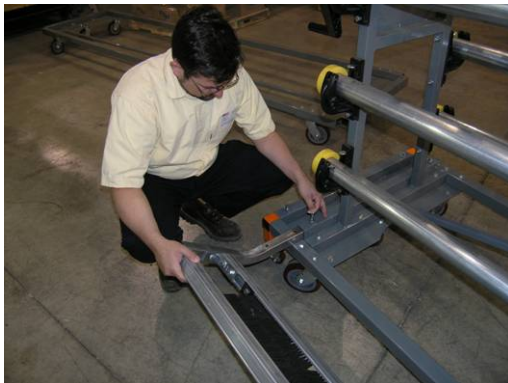
Fig. 18.2 Slide Brush Assembly into Position
